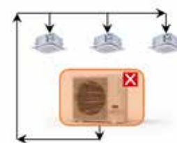
Refrigerant stored in IDU
