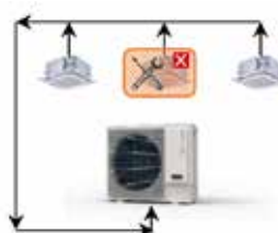
Refrigerant stored in ODU
