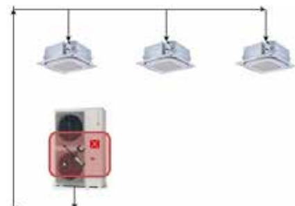
Refrigerant stored in IDU
