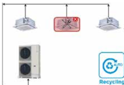
Refrigerant stored in ODU
