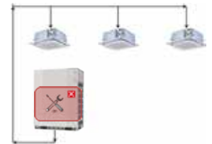
Refrigerant stored in IDU
