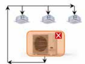
Refrigerant stored in IDU
