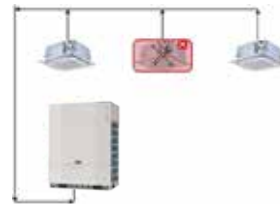
Refrigerant stored in ODU
