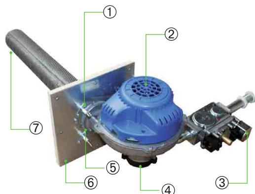
The **premix burner group** is modulating and with a wide regulation range, from 100% to 30%. The gas valve delivers the fuel in relation to the combustion air flow rate pre-set by the manufacturer. The high pressure available at the chimney satisfies all the requirements relating to installation and configuration of the flue gas exhaust ducts and combustion air intake.
