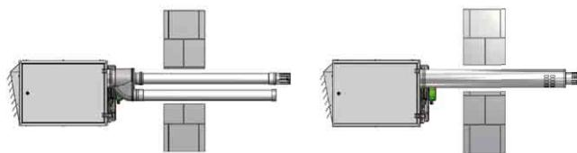
The gas appliance must be connected to a single duct that brings combustion products to the outside of the room. The combustion air is taken directly from the appliance installation area.
