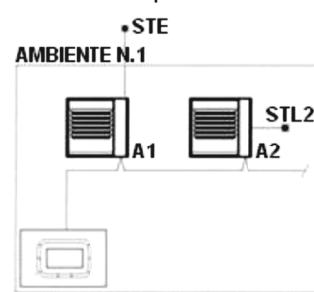
Both devices are controlled by a single remote control panel with the difference that **A2** is equipped with a local temperature probe **STL2** (optional) that communicates with the remote control panel for dedicated power modulation. Moreover, the external temperature probe **STE** (optional) allows for the maximum output power of both units to be adjusted.
