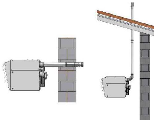
The gas appliance must be connected to a single duct that brings combustion products outside of the room. The combustion air is taken directly from the appliance installation area.
