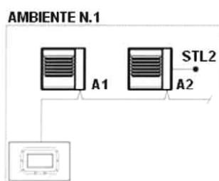
Both units are controlled by a single remote control panel with the difference that **A2** is equipped with a local temperature probe **STL2** (optional) that communicates with the remote control panel for a dedicated power modulation.
