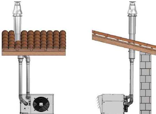
The gas appliance must be connected to two ducts, one for the discharge of the combustion products and the other for the intake of combustion air with a coaxial terminal communicating with the environment outside the installation environment, from the roof.
