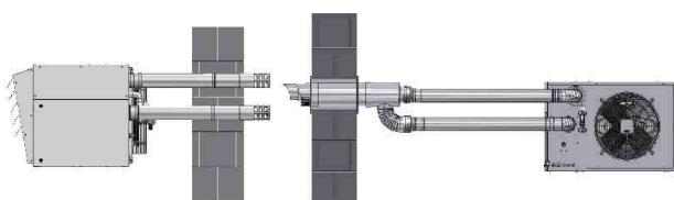
The gas appliance has two ducts, one for the discharge of the combustion products and the other for the intake of combustion air, both communicating with the environment outside the installation room. The outlet must be wall-mounted with two separate ducts or with two coaxial ducts.
