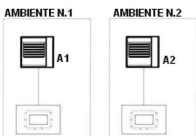
Standard solution without additional temperature probes.
