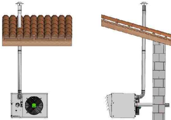
The gas appliance must be connected to two separate ducts communicating with the outside. The one to discharge the products of the combustion through the roof while the other one for the combustion air intake through the wall.
