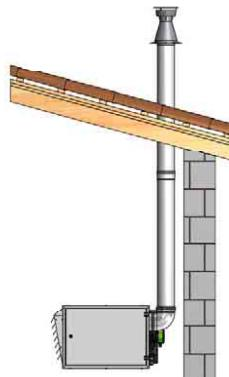
The gas appliance must be connected to two separate ducts communicating with the outside. The one to discharge the products of the combustion through the roof while the other one for the combustion air intake through the wall.
