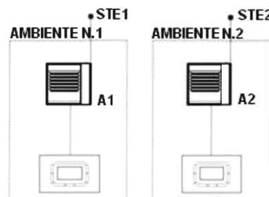
Solution with external temperature probes STE1 and STE2 (optional).
