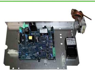
**Multifunction electronic board** that provides the functions of ignition of the burner, flame monitoring and total safety.
