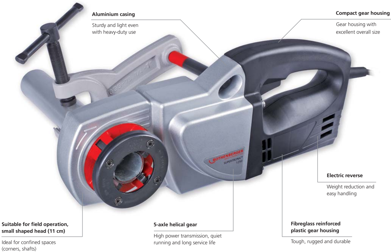
Compact design, only 4.9 kg, ideal for portable operation
