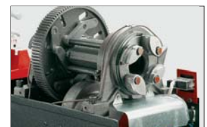
SUPER GRIP pipe chuck system
