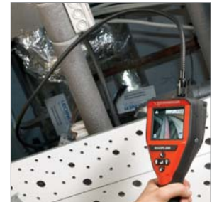
Camera head with high-performance LEDs
