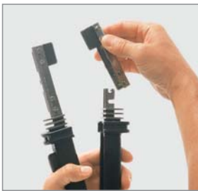
Simple replacement of electrodes and electrode holders
