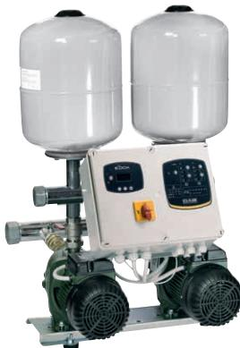
Booster set with 2 EURO centrifugal pumps complete with baseplate, suction and delivery manifold, 2 membrane vessels and control panel supplied complete with:
