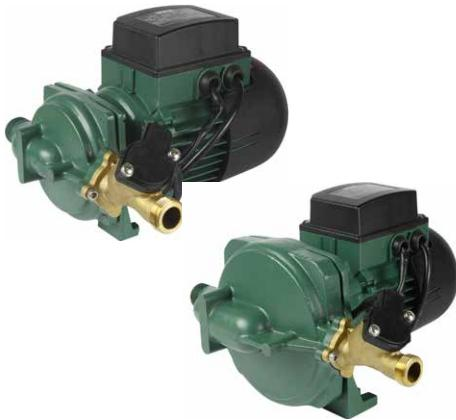
K-HA single impeller centrifugal pump is designed for water pressure boosting in households, flats (domestic properties) to provide additional pressure to hot and cold water taps and similar outlet points. K-HA centrifugal pump is mainly for use in open vented systems(tanks), but may also be installed directly on the incoming water mains supply to feed a boiler, provided approval has been obtained from the local Water Company. The pump is supplied with a 0,3 meter power cable.
