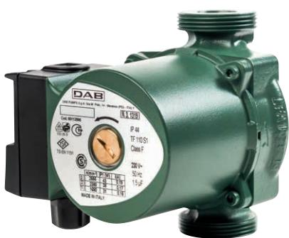
Single body consisting of a cast iron hydraulic unit. Die-cast aluminium motor casing. Technopolymer impeller. Tempered stainless steel driving shaft mounted on graphite brushings lubricated by the pumped liquid itself. Stainless steel protective rotor sleeve, stator sleeve and closing flange. Ceramic thrust bearing, E.P.D.M. O-rings and brass air outlet cap. The two-pole asynchronous motor with wet rotor is self-protected for resistance.
