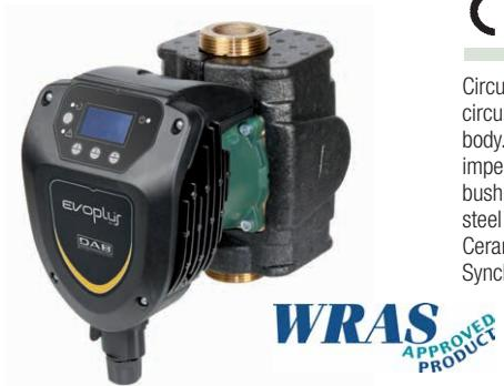
Circulator for domestic hot water systems of the closed circuit pressurized type or open circuit type. Bronze pump body. Motor casing in die-cast aluminium. Technopolymer impeller. Ceramic motor shaft mounted on graphite bushings lubricated by the pumped liquid. Stainless steel rotor sleeve, stator sleeve and closing flange. Ceramic thrust ring, ethylene propylene sealing rings. Synchronous motor with permanent magnet rotor.
