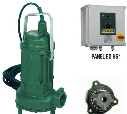
Submersible pump with cast iron pump body, motor casing and adjustment ring impeller. Grinder device in micro casting steel. Stainless steel shaft, handle, filter, bolts and screws. Silicon/carbide mechanical seal, inspectionable oil chamber.
