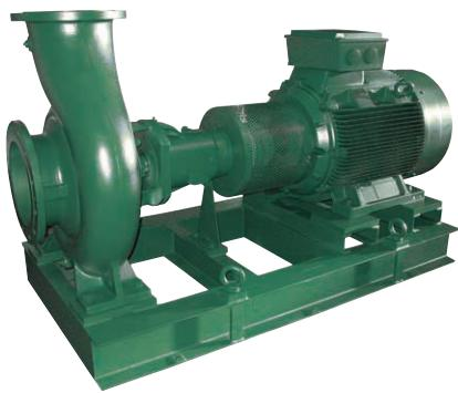
Single-stage centrifugal pump body with axial suction port, radial discharge port and horizontal shaft components. The KDN pumps have dimensions and nominal performances according to EN 733 (10 bar) but are designed for 16 bar operation wherever the shaft seal type allows it.
