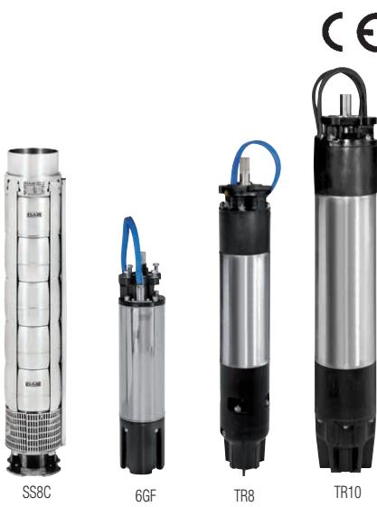
Multistage mixed-flow borehole electric pumps, completely made in stainless steel (AISI 304L or AISI 316 on request), usable for wells from a minimum diameter equal to pump size or greater and capable of developing a wide range of Flows and Heads.
