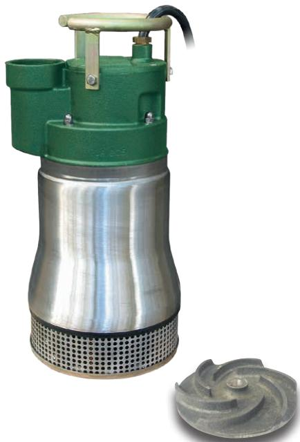
Submersible electric pumps particularly suitable for the removal of drainage water in construction sites, open mines or quarries. Thanks to their rugged construction and reliability, these pumps can be used with harsh and abrasive liquids containing solids with maximum dimensions of up to 6 mm.
