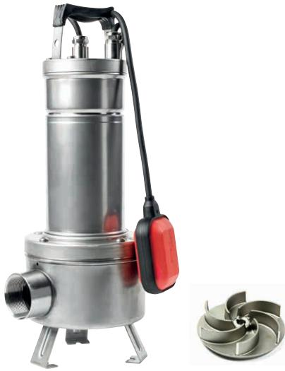
Submersible centrifugal pump with liquid vortex cast steel impeller, suitable for pumping sewer water and waste water in general containing solids up to a maximum size of 50 mm.
