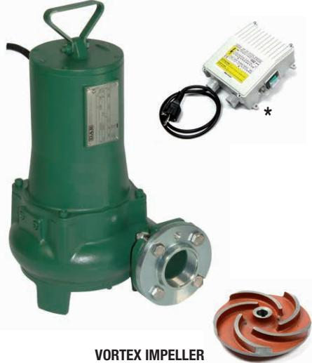
Cast iron submersible pumps vortex impeller for sewage, suitable for foul waste water with solid contents with **42 mm** as maximum diameter. Technopolymer upper cover with handle. Motor body, hydraulic section and any impeller in cast iron EN GJL 200.
