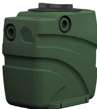
Automatic collection and lifting stations. Ideal for the collection and pumping into the sewer network of dirty and domestic drain waste water from underground locations below the level of the sewer network. FEKABOX 110 consists of a polyethylene tank with an effective capacity of 110 litres, with cover fitted with plastic seal.
