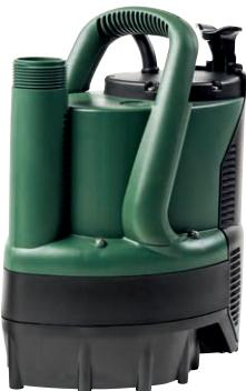
Submersible pumps specifically designed for uses in narrow pits with dimensions down to 20 cm x 20 cm. Suitable to pump clear water containing particles with maximum diameter up to 5 mm.
