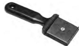
The Stabi-Pipes are finished with an aluminium coating on their outer surface. This aluminium coating has to be scraped off within the welding section before welding the pipe. Each peeling tool is designed for two individual pipe diameters. The peeling tools for diameters from 50 mm on have turning handles.
