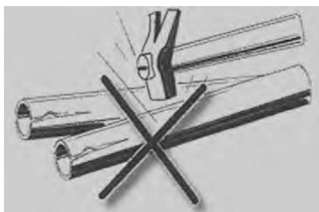
At temperatures lower than 0° prevent impacts (especially against pipe ends), excessive loads, crushing or bending. Please handle pipes with care at low temperatures.
